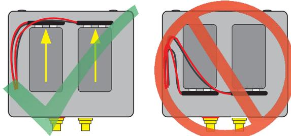
Reconnect the battery snaps to the new batteries. It does not matter which snap is connected to which battery. Place the batteries in the holders. Replace top cover using care not to pinch any wires. Reinstall the four screws.
